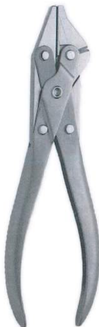
Flat Nose Plier MB9-637 18.5 cm 7 1/4" parallel grip, incorporated cutter, for hard wires up to 1.6 mm
